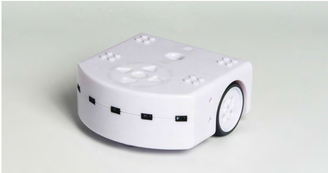
Figure 4.1 – The Thymio II robot is a small wheeled robot for children (image courtesy of Association Mobsya).
