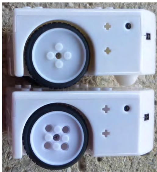
Figure 4.6 – The new wheel (down) has additional Lego technics holes to facilitate the transmission of rotation.
