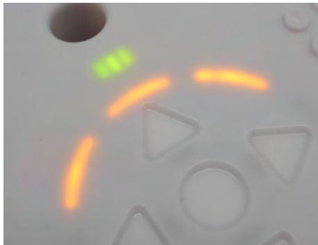
(a) LED diffusion delimited with a waveguide. These LEDs are placed 16 mm away from the plastic cover.
