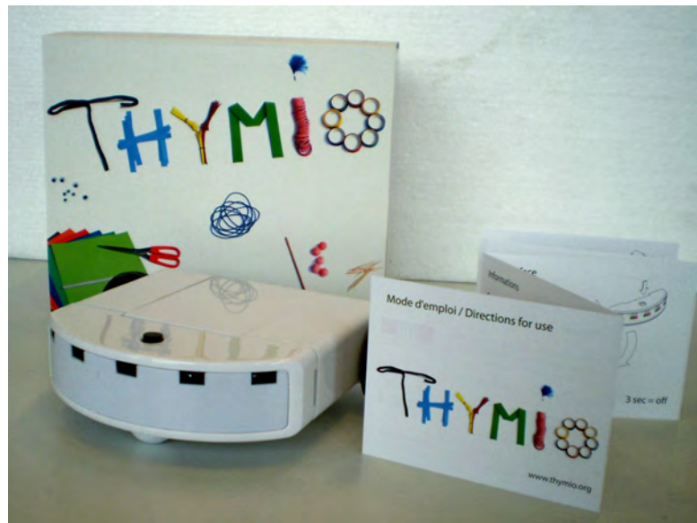
Figure 3.8 – The produced version of Thymio. Some details were modified when setting up the production: the front plastic part was changed to translucent white to show the LEDs and holes were added for the IR sensors. The attachments changed slightly.
