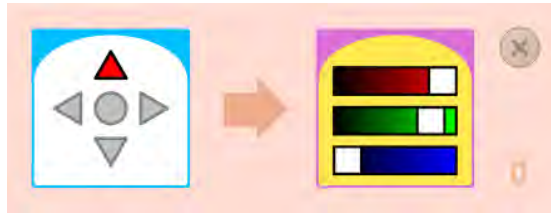
Figure 5.2 – An event-action pair. Here the Forward button was pressed event is associated to Body LEDs display colour yellow action.
