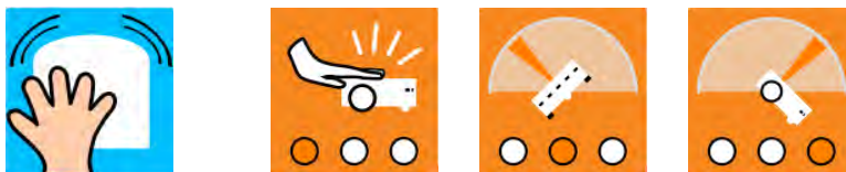
Figure 5.13 – Accelerometer (tap) event block, 1.3.1. version (right). On the left, the future advanced version, with three variants: shock, pitch or roll detection.
