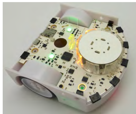
(d) The waveguide, touch PCB and main PCB are assembled separately. The motors and battery are connected to the PCB which is placed on top, all IR sensors fitting in the spaces provided. Finally the top case is screwed in place, after plugging the loudspeaker.
