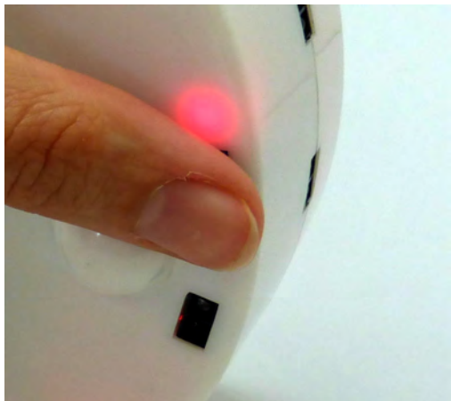
(a) The finger in front of the bottom sensor lights up the LED.
