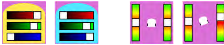
Figure 5.3 – The blocks are animated to reflect the settings chosen by the user. On the left, two configurations of the top colour action: depending on the positions of the sliders representing the Red, Green and Blue values, the background colour changes. On the right, the motor action block as it animates: in one case both sliders representing motors speeds are in the middle, the robot does not move, in the other case, both sliders are on a forward position, the right one higher, so the animate robot on the block turns left.
