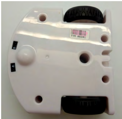
(a) Bottom of Thymio II. One can see the two ground IR sensors, the slider ball, the four screw holes, the pencil support hole and the trailer hook.
